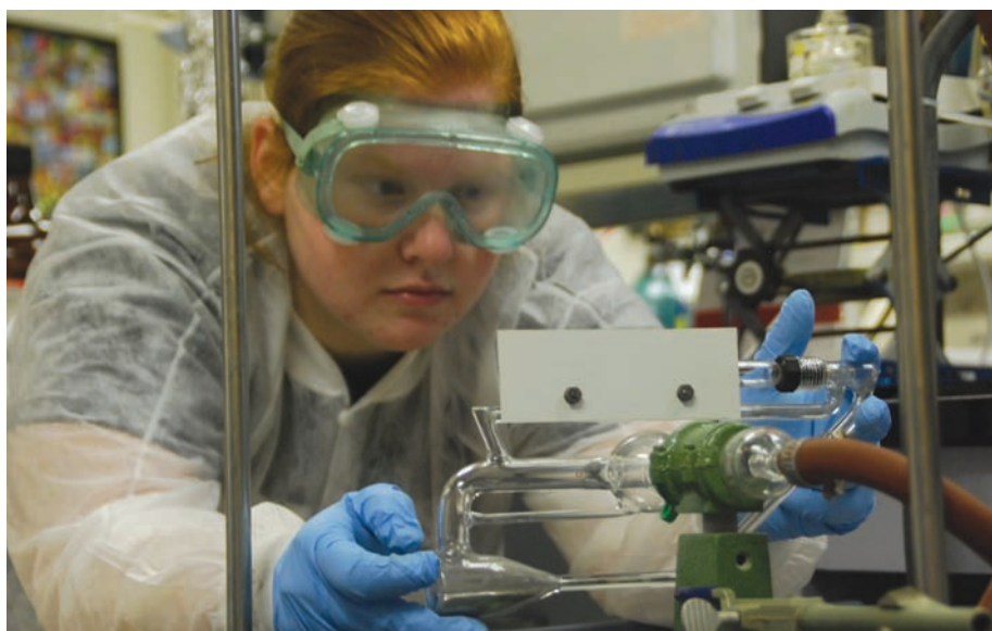
Student researcher Lisa Pagano uses a monometer to measure the pressure during a fractional distillation.
